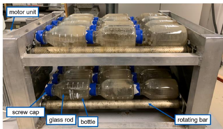
Figure 2: Rolling Bottle Test Setup
