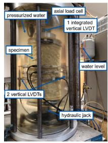
Figure 1: RLTT Specimen Setup
