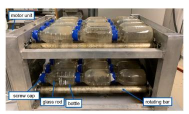
Figure 2: Rolling Bottle Test Setup
