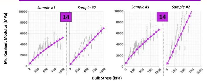
Figure 7: Soil Sement EF (ACE-B) Resilient Modulus (M<sub>R</sub>) before (left) and after (right) 10 Freeze/Thaw cycles
