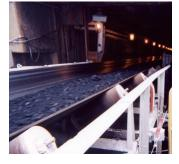
So-Long is a polymer-based emulsion in an easy-to-apply liquid form which provides both short and long term dust suppression when loading and transporting railroad ballast.
